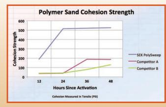
**COHESION** PolySweep achieves superior cohesion versus the competition by a factor of 6 (180 psi VS 30 psi) within 12 hours of activation. PolySweep maintains superior cohesion performance at 24, 36, and 48 hours after activation. (See chart.)
