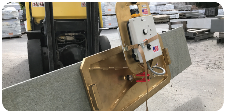
ES Power Pack with the ES Housing Unit and ES Pad Size 18" x 36"
