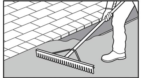
**Step 1:** Prior to compacting the pavers or natural stone, remove bedding layer (sand or chips) that extends outside the perimeter. For optimal performance, remove all of the bedding material down to the base material.
