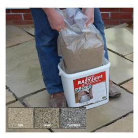
**EASYJoint** is a quick, effective and aesthetically pleasing All Weather Jointing Compound designed to be applied over wet surfaces, while filling joints between paver stones, natural stone (super wide joints up to 5"), concrete flags and clay pavers. It is ideal for permeable applications and is suitable for all types of paving material provided there is a gap of at least 3mm wide and 25mm deep.
