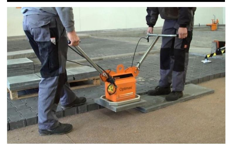
This suction device is perfect for lifting and installing of dry-cast and wet-cast stone between 210 - 440 lbs. It is equipped with two adjustable handles and a standard eye-bolt that can be attached for machine operation.
