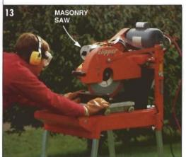
CUT PAVERS on masonry saw. Saw has a built-in sliding carriage for moving pavers past the blade. Recirculating water keeps blade cool and lubricated.
