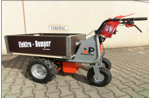
transport platform with adjustable width load carrying beds 90x79x26cm / 35"x31"x10"
