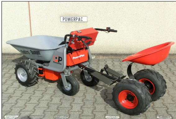
Seat with spring borne, foot service brake and adapter
