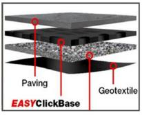
1. Excavate 1" bedding layer + 1" **EASYClickBase** + Depth of stone used at a 2-5% pitch. Don't over excavate.
