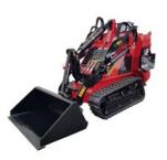
Payload: 660 lbs. **Size** Overall Width: 38.4" Overall Length: 8'3" Weight: 2315 lbs. **Engine** Honda GX 690 3600 RPM 18.4 kW / 25.0 hp 2 Cyl. / 4-stroke Electric Start
