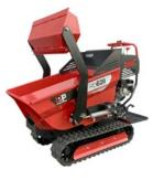
Capacity Volume: 0.4 Cu. Yard. Payload: 1367 lbs. Size Overall Width: 33.1" Overall Length: 72.4" Weight: 849 lbs. Engine Honda GX 200 3600 RPM 6.5 HP
